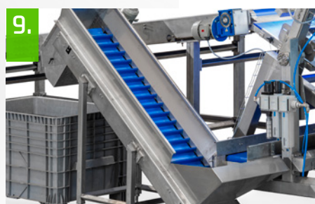
Belt hopper for the handling of the non-compliant products in a dedicated bin.
