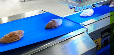
SENSURE STARGATE SL-C is an innovative vision system that, thanks to the use of SENSURE SYNAPSE technology, allows you to perform the quality control of highly variable products and automatically reject non-compliant ones. SENSURE STARGATE SL-C also guarantees continuous monitoring of the process with data collection and analysis, providing a realtime display and dedicated reporting.
